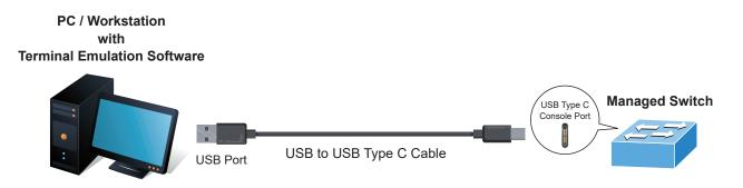
Figure 4-1: Industrial Managed Switch Console Connectivity
